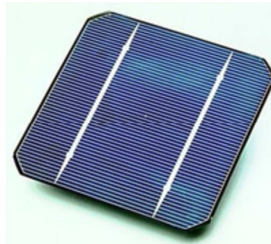
Figure I-19 : cellule photovoltaïque monocristalline.
