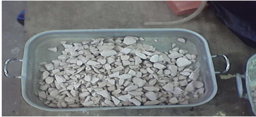
Figure III.19. La brique silico_calcaire concassé
