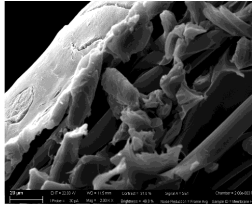
Figure 37. Structure de la membrane HL
