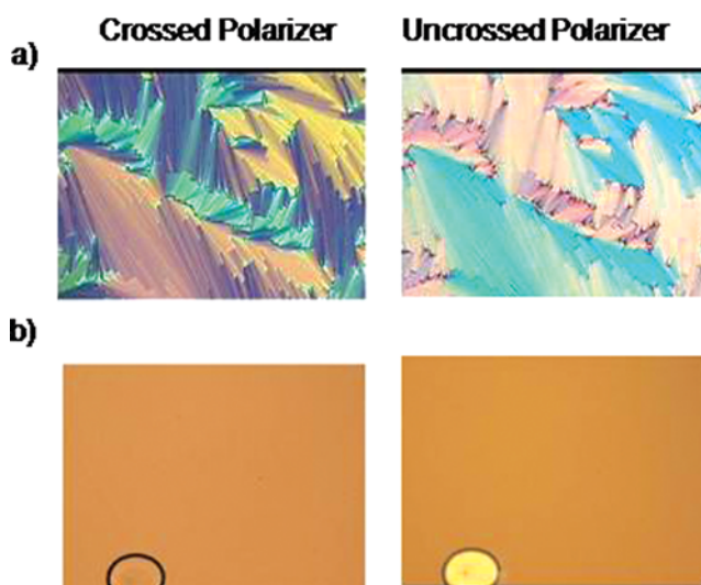
Figure 1. Optical micrographs observed at T=25^{\circ}\text{C} under crossed and uncrossed polarizers for a) pure 8CB and b) pure dPS. The ellipsoidal object in the latter case corresponds to an air bubble used as reference. (Figure appears in color online.)
