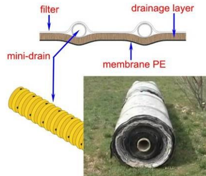
Figure11. Structure of the geocomposite DRAINTUBE FT/PE
