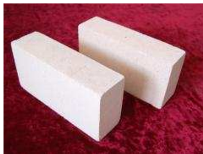
Figure 1.12 Brique silico-calcaire (POURRAT, 2009)
