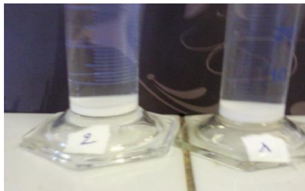
Figure III.7 : Test de sédimentation de PG100-St100, 1 :2ml; 2 :5ml de solution 30%
