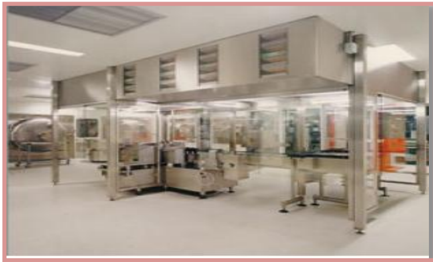
Figure 12 : Flux laminaire verticale [20]
