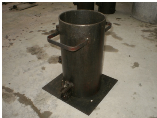
Figure 2. 2 Moule cylindrique 16x32 (cm)
