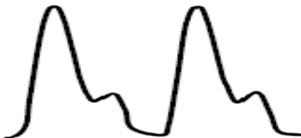
Figure I.22 - Forme de signal PPG [14]
