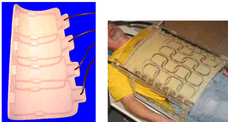
Figure I.18 : Antenne 'phased array'
