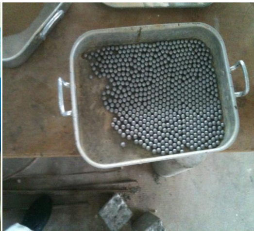
Figure 3. 7 La machine de micro-Deval Figure 3. 8 Les billes de la machine
