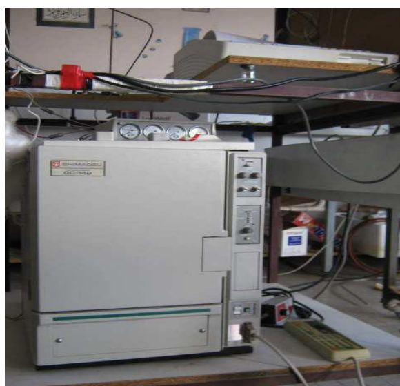
Figure 13: Chromatographe Shimadzu GC-14 B.
