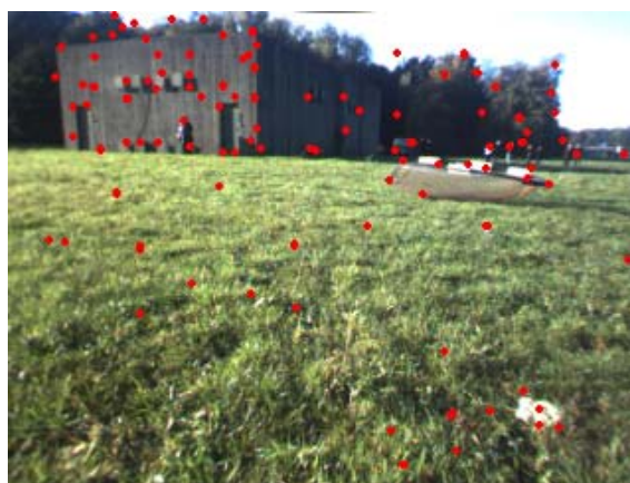
Fig. 2. Features detected using the SIFT algorithm.
