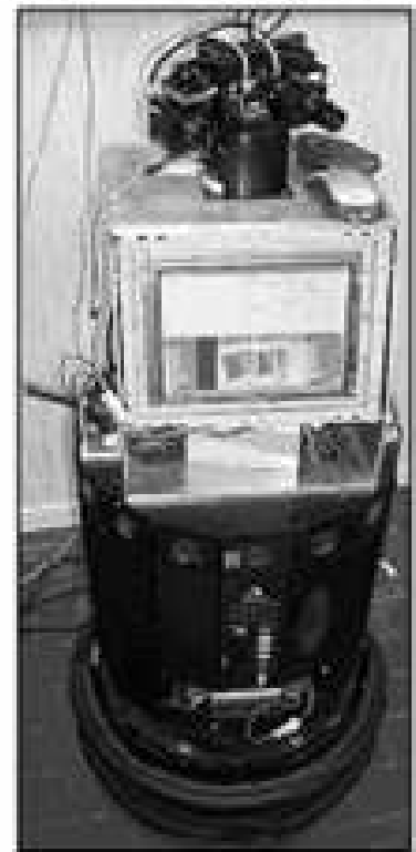
Figure 3. The Nomad200 robot with the upper PC-platform and the biclops head on top. The stereo vision system forms the robot's eyes
