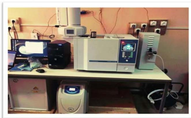
**Figure 4.** Appareil CPG.
