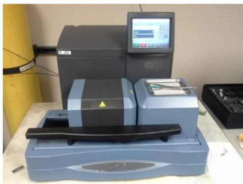
*Figure I-4: Appareil ATG-DSC SDT QS600 C.R.A.P.C*
