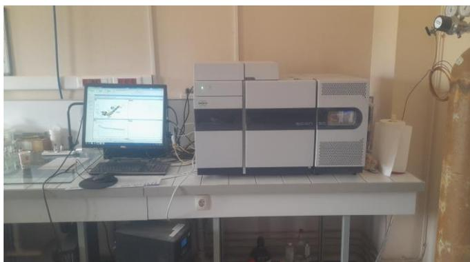
*Figure I-1: Dispositif GC-MS Bruker SCION 50 (LCSCO)*
