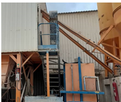
Figure 1.21: Endless screw conveyor connected to the mixer Figure 1.22: Endless screw conveyor structure
