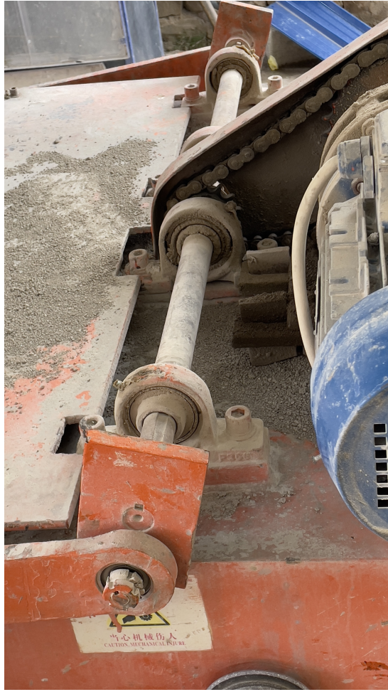
Figure 2.5: Timing chain that connects the motor with the mixing cart
