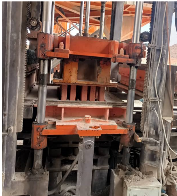
Figure 1.15: the machine applying pressure
