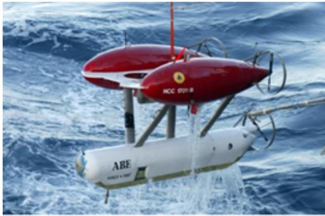
FIGURE 1.16 – Sous-marin AUV (ABE) [13]
