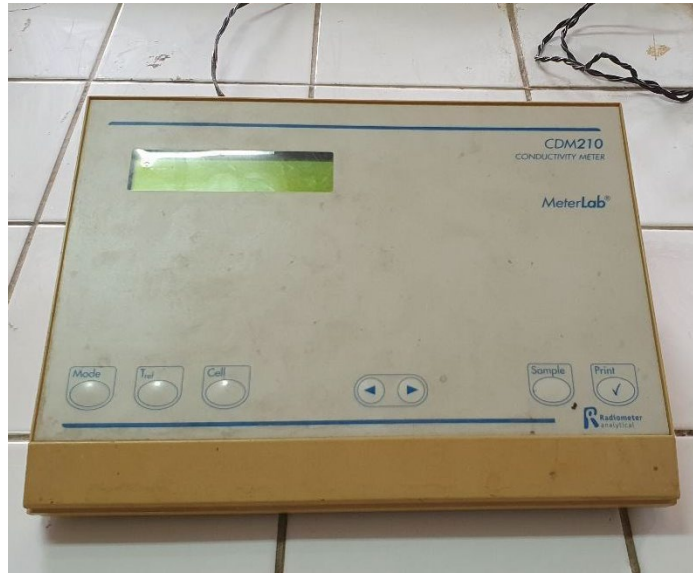
Figure II.5. Conductivity meter device CDM210 (LAEPO).
