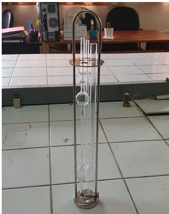
Figure II.6. U-tube viscometer (LAEPO).
