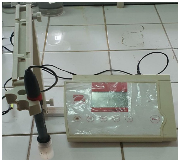
Figure II.4. Potentiometer device OHAUS STARTER 2C (LAEPO)
