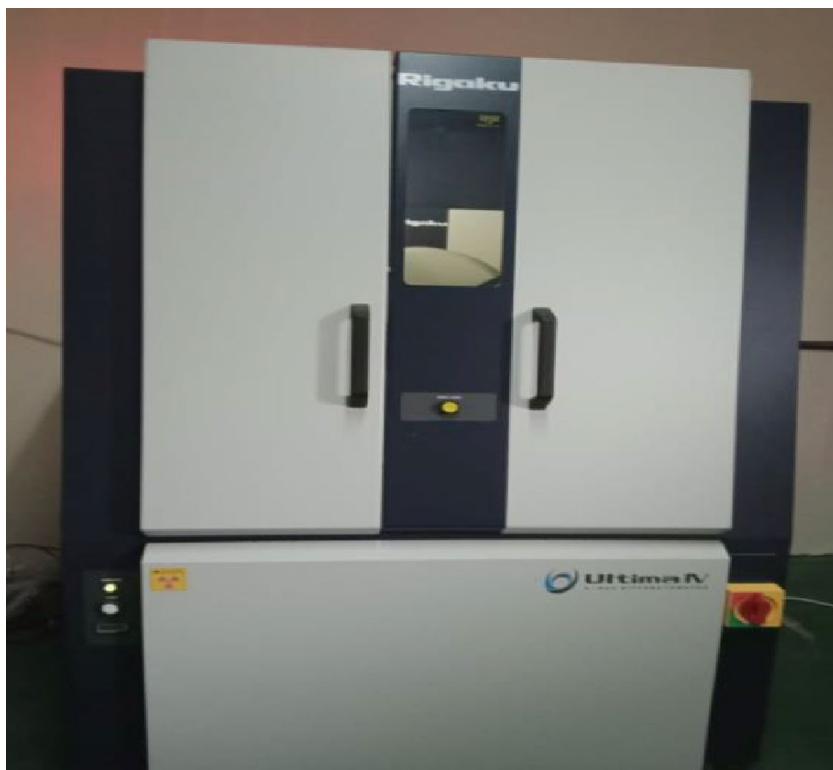
Figure II.3. X-ray diffraction apparatus.
