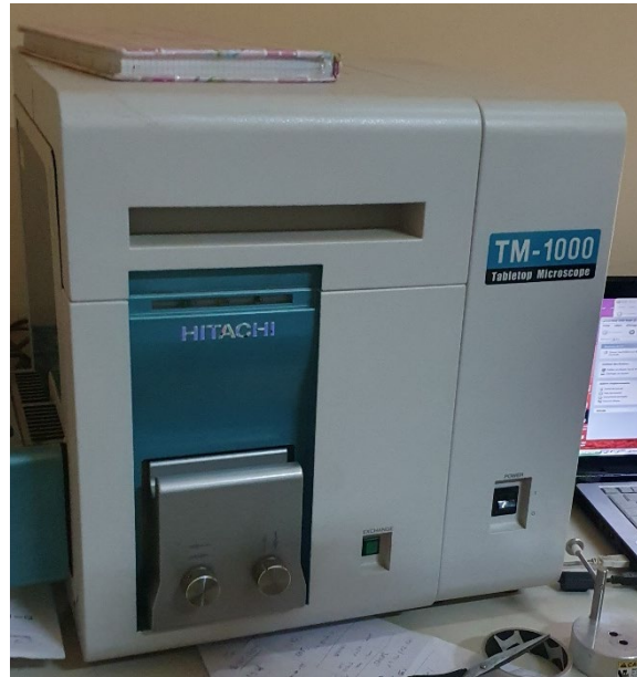
Figure II.9. Scanning Electron Microscopy (SEM) TM-1000.
