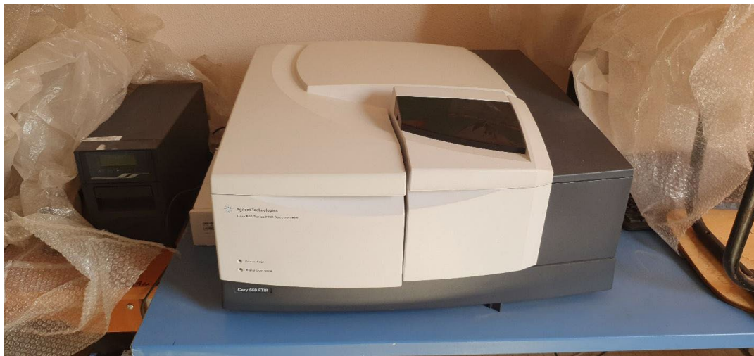
Figure II.2. Infrared Spectroscopy (CARY 600 SERIES).
