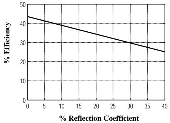
Fig. 2: Efficiency variation of solar cell with respect to reflection coefficient.
