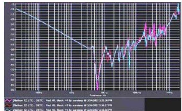
Figure 12 : HV winding response (LV short)
