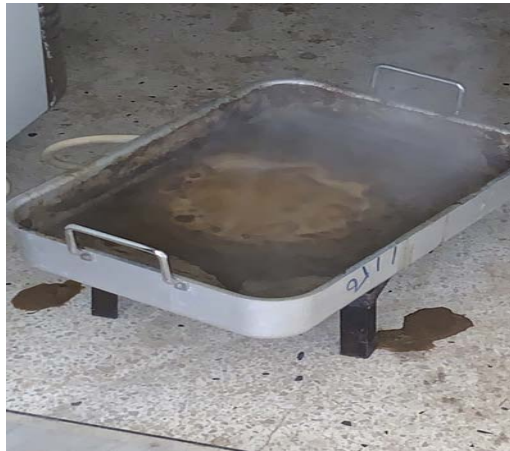
Image 21: Manure solution being sterilised by heating (original photo)
