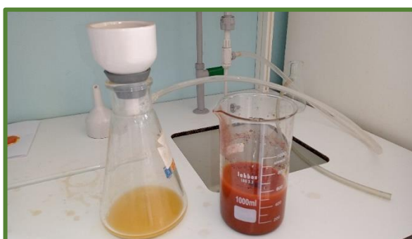
Figure 67: Montage de filtration.
