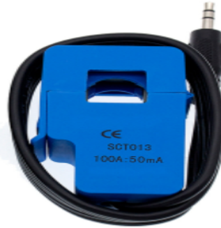
FIGURE II.2 – Transformateur de courant 100A/50mA
