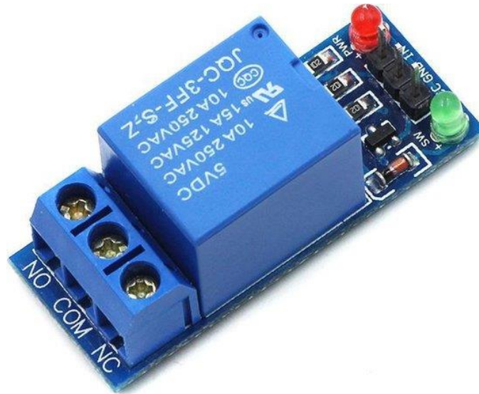
Figure 2.28 Type module Relais 5 V Arduino[33].
