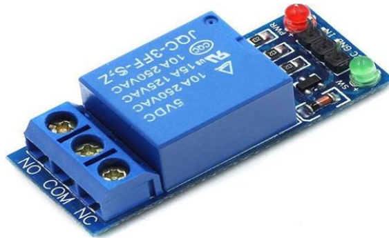
Figure III- 10: Module relais 5V1 canal
