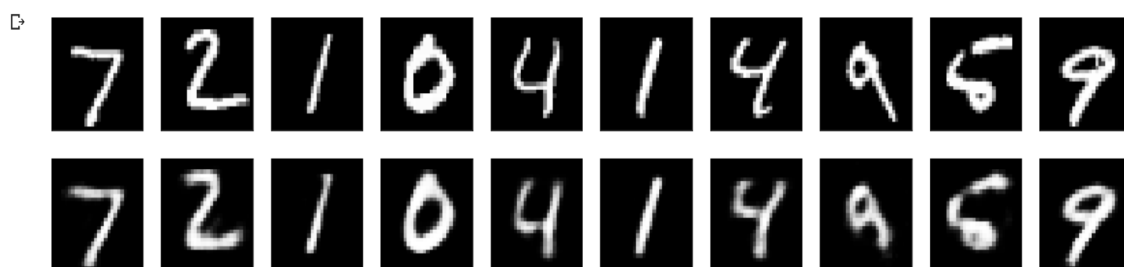
Figure 2.11: Result of the stacked AE, The top row is the original digits, and the bottom row is the reconstructed digits.
