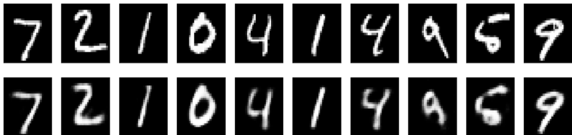
Figure 2.8: Result of the sparse AE, The top row is the original digits, and the bottom row is the reconstructed digits.
