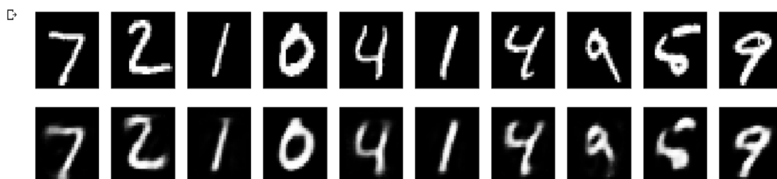
Figure 2.3: Result of the simple AE, The top row is the original digits, and the bottom row is the reconstructed digits.
