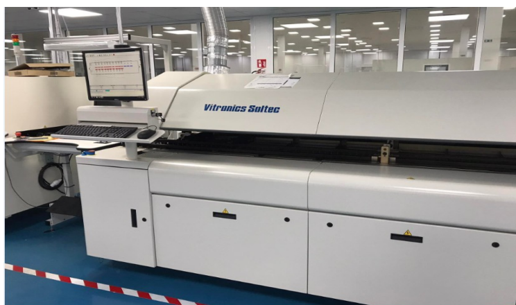
Figure II.6 : Four à refusion industriel [6].
