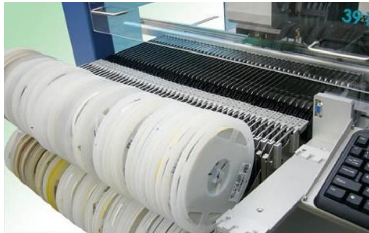
Figure I.3. Pose des composants CMS [3].
