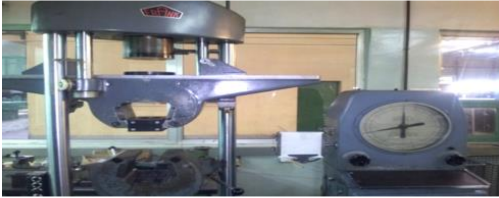
Figure III. 41: La machine d'essai de traction. [22]
