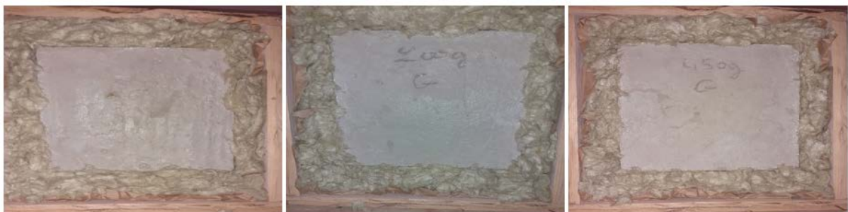
Figure III. 6: Les différents panneaux de la chape : (a) chape ordinaire, (b) chape/diatomite (gravier 200g), (c) chape/diatomite (gravier 450g).
