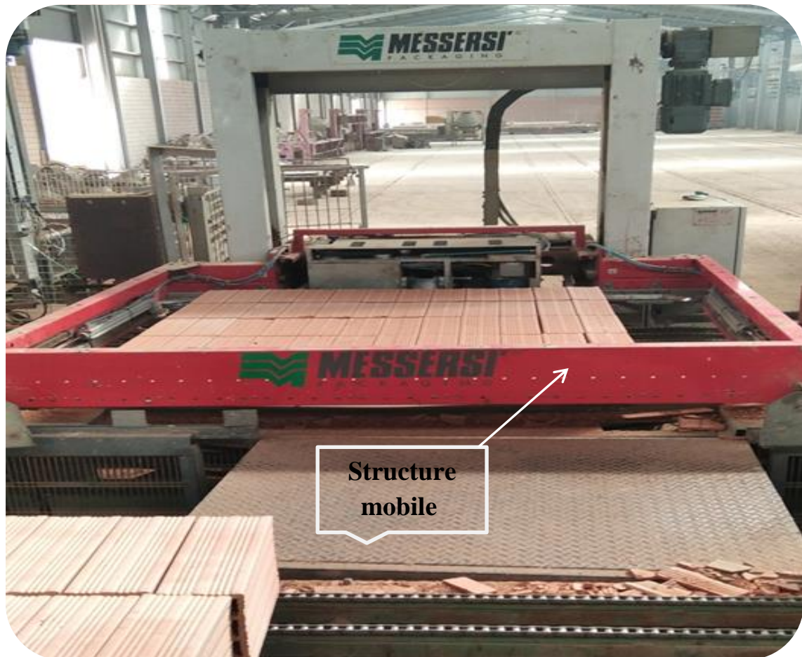
Figure 2-12: Structure métallique mobile
