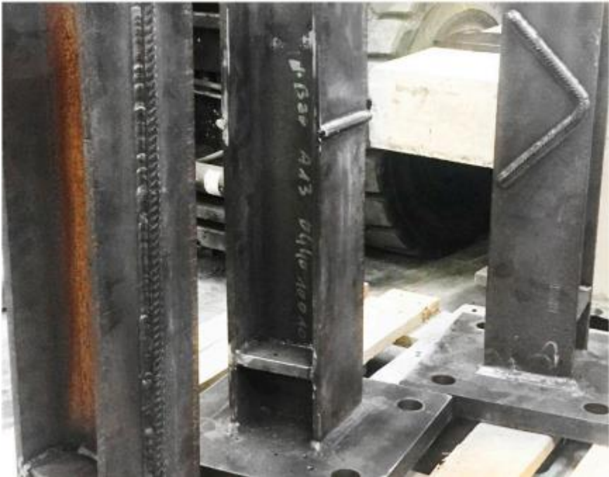
f) Transversal connector, angled, V-shaped connector and longitudinal connector [16].
