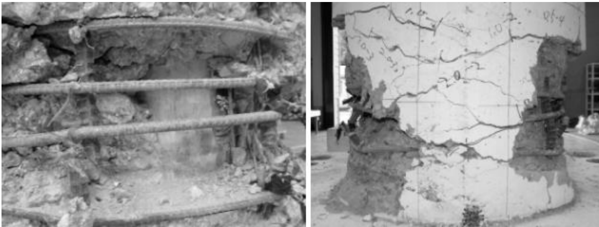
b) Composite column with 4 steel tubes
