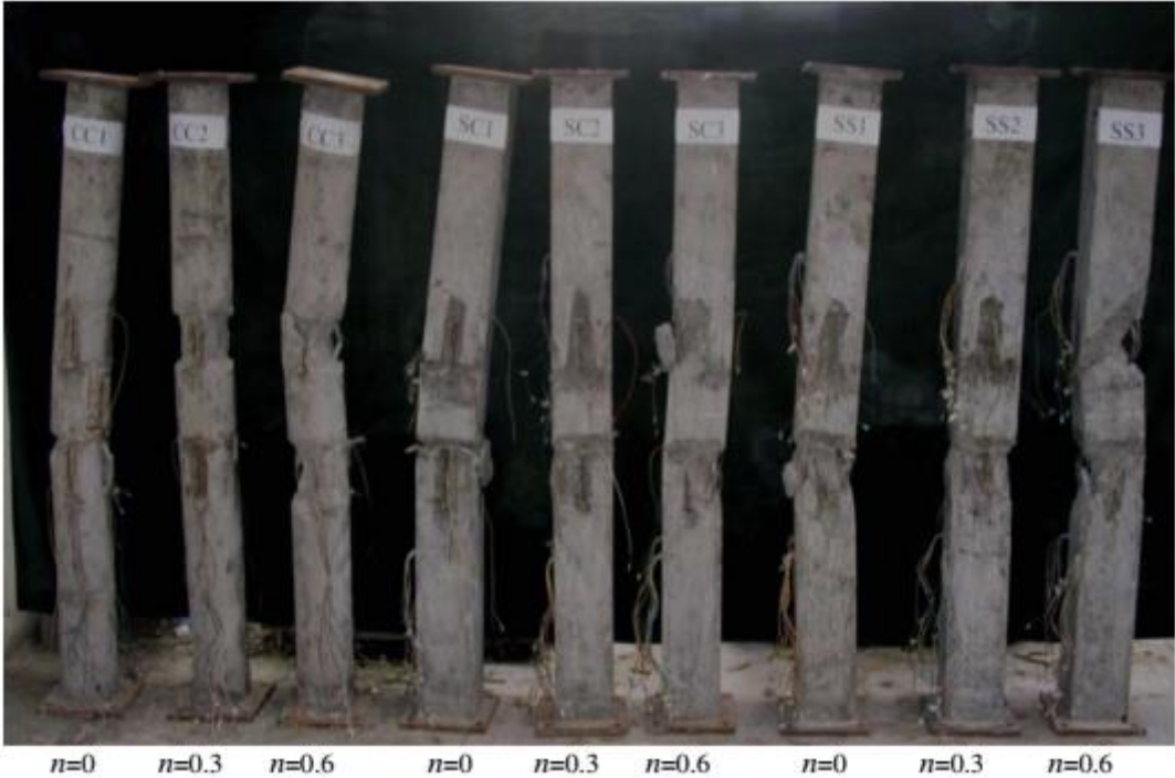
Figure I.12: CFSTRC columns after tests [30].
