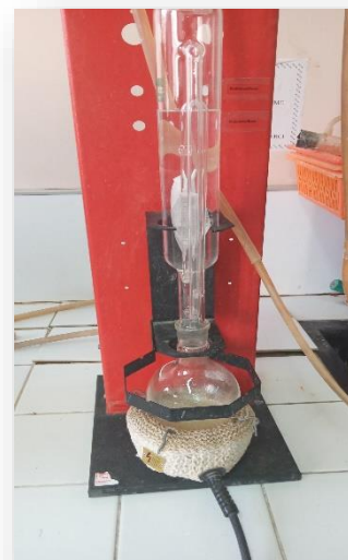
Figure 16: montage du Soxhlet
