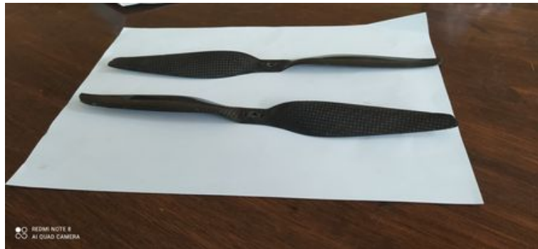
Figure 5.5: 10 inch carbon fiber propellers.
