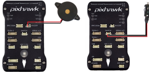
Figure 5.8: buzzer and safety switch-pixhawk connection
