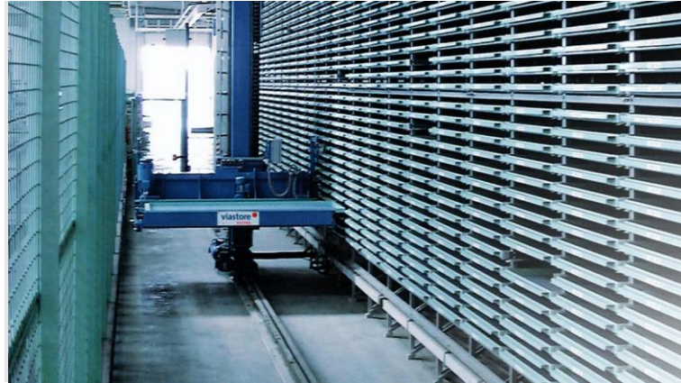
Figure I.2 Machine de stockage/déstockage [5]
