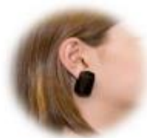
FIG. 3. Wireless PPG sensor attached to the earlobe.
