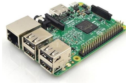
Figure IV. 6 Carte Raspberry Pi 3 Type B
