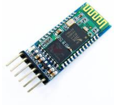
Figure II.12: Module Bluetooth hc-05.
