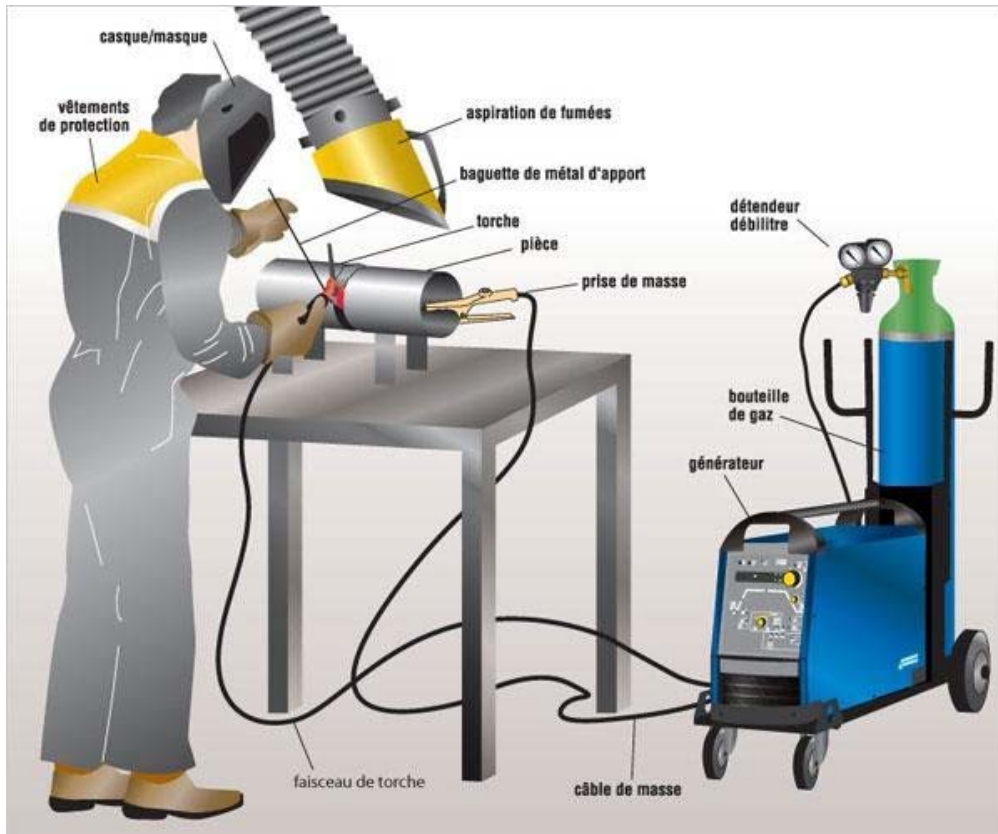
Figure 1-17 : Installation de soudage TIG [8].
