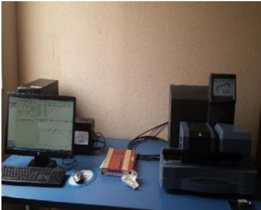
Figure II.6 : Appareil TGA (TA Q600)
