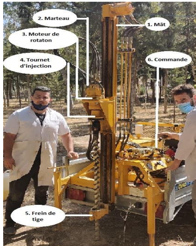
Figure 3-10 Architecture de machine de forage Sedidrill S80.
