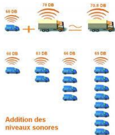
Figure 1-9 : Addition des niveaux sonores. [11]
