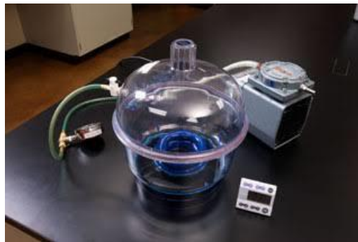
Figure 13: Bell shaped chamber connected to a vacuum pump (42)
