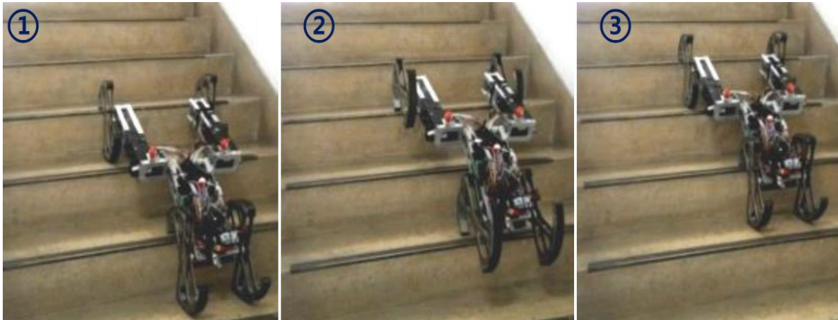
Figure II.10 : Robot Claw-Wheel à transformation hybride.
