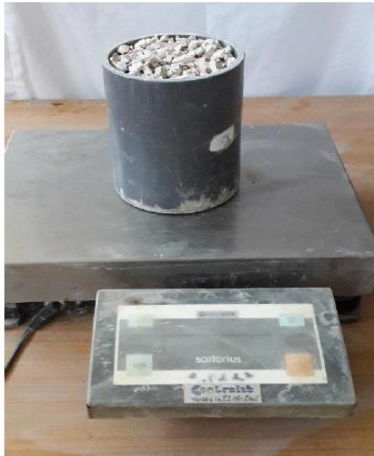
Figure IV.5: Test to measure apparent density
