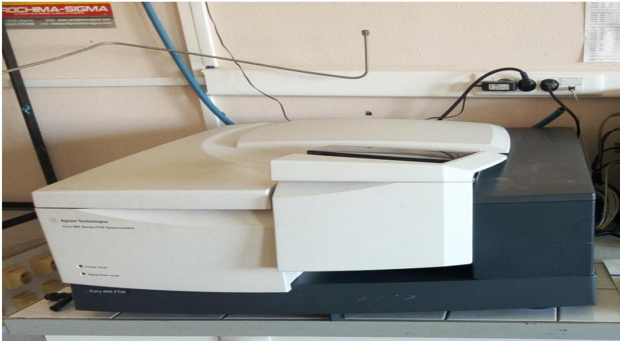
**Figure II.4:**Appareil FTIR Agilent Technologies Cary 600 series.
