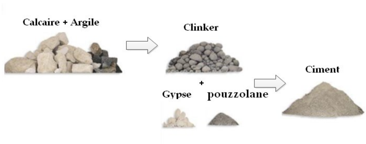
Figure 1.3 Composants du ciment
