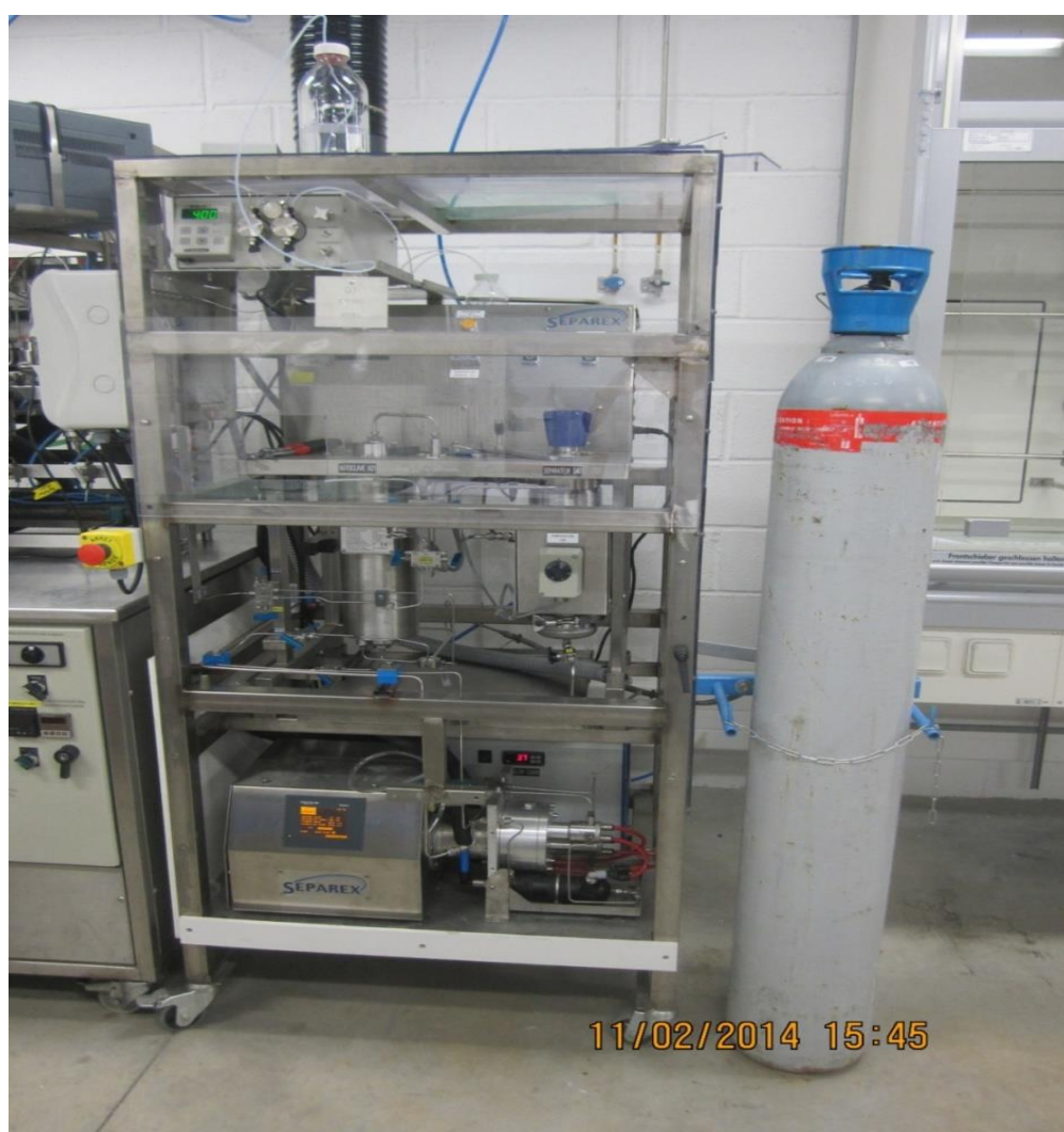
Figure II.5: Installation d'extraction supercritique «SFE1000 bar»
