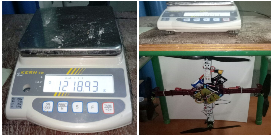
FIGURE III.27 – Le poids du quadrirotor
