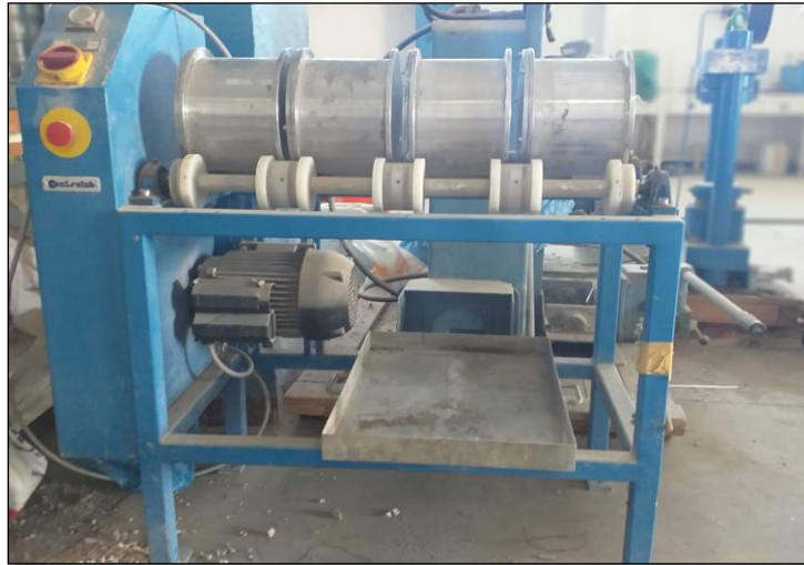
Figure III.13 : L'essai de Micro-Deval
