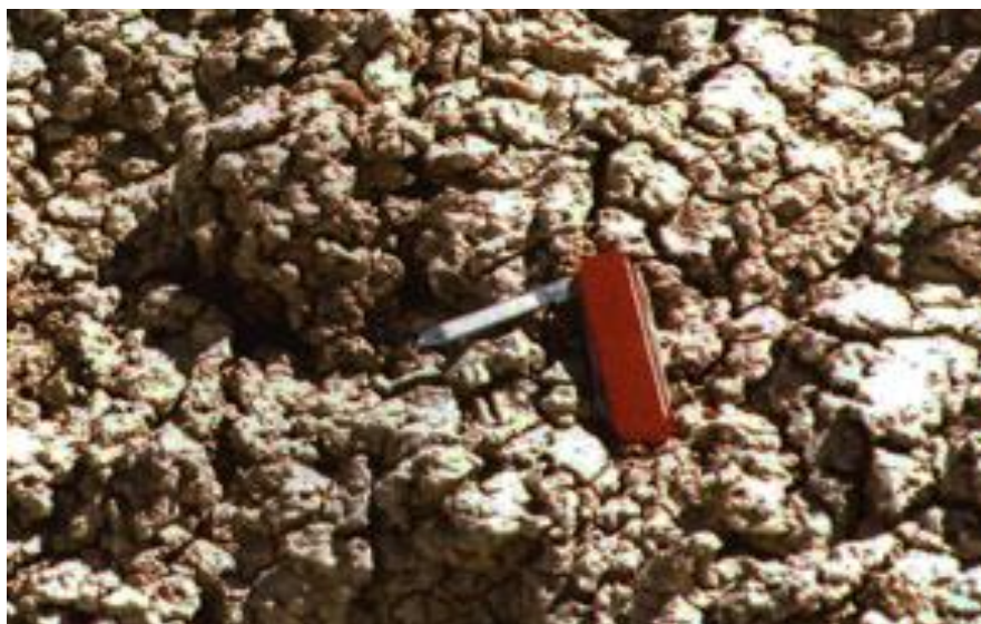
Figure I-2 : sol expansif montrant du "Pop-corn" (THE UNIVERSITY OF ARIZONA, 2019 ).
